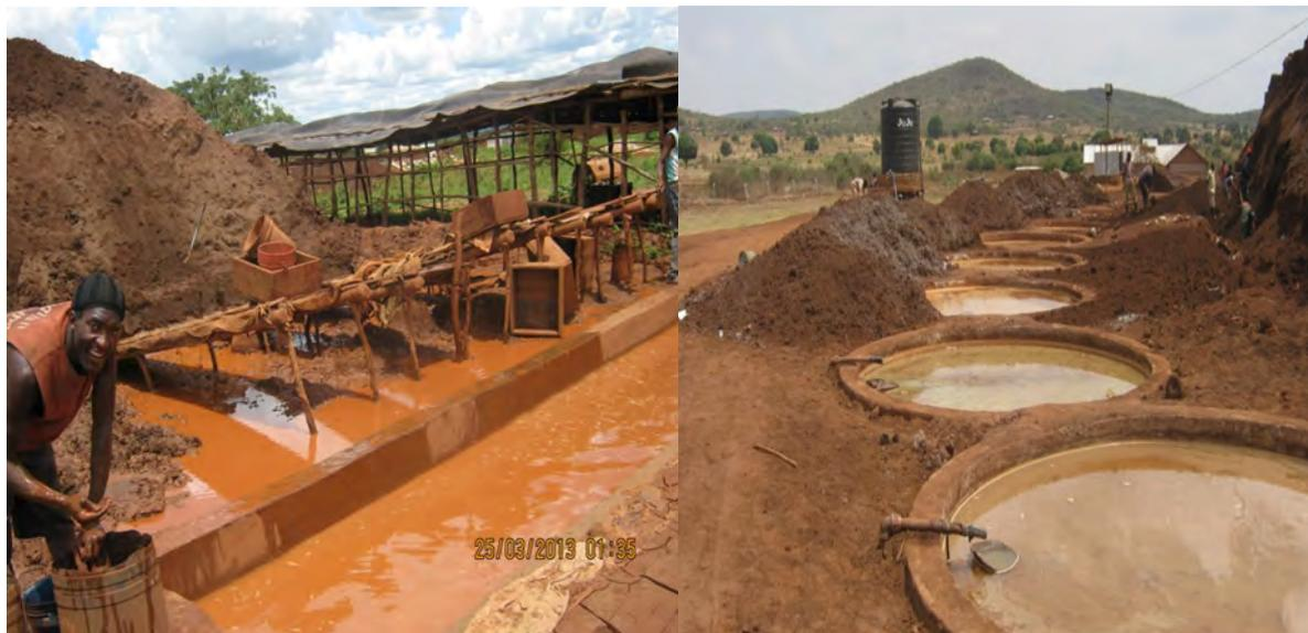
Plate 10-3: Small scale Gold mining activities in Misungwi and chemical spillage (Cyanide Chemicals) in one of the Vat processing plants in Chunya DC
